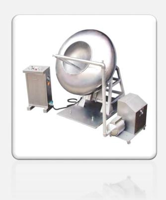
Coating Machine is available with 12", 24", 30", 36", 42", 48", 60" or 72", size SS Pan. Coating Machine is totally enclosed with MS Cladding with standard Gear Box, Motor, Hot Air Blowing arrangement. Machine is designed with MS fabricated structure and all arrangement – except electric control, air filter and SS Pan are inside the enclosure, which makes simple cleanable outside covering.
